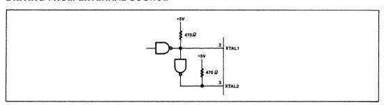
XTAL 1 MUST BE HIGH 35-65% OF THE PERIOD AND XTAL 2 MUST BE HIGH 35-65% OF THE PERIOD. RISE AND FALL TIMES MUST NOT EXCEED 20ns.
